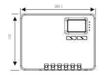
Product Size: 280.1\*210.1\*90.6mm Installation Size: 256\*154.5mm Installation Holes Diameter: φ2.5 & φ5 Connection Holes Size:7.5\*7.5mm
